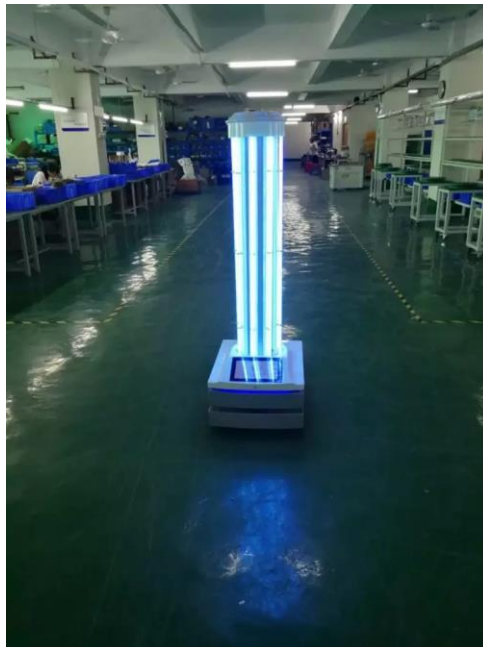
Figure 1. Autonomous UVC Disinfection Robot (SIFROBOT-6.53.) To ensure safety, the robot's body includes a human body detection module. During operation, the ultraviolet light automatically shuts off upon detecting a human presence, preventing harm to people.
